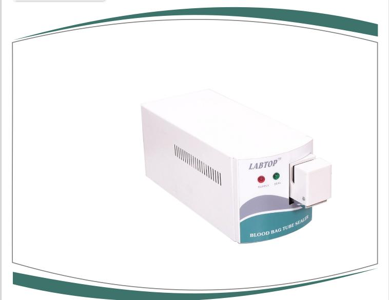
**The LABTOP** ® Blood Bag Tube Sealer is a compact equipment to seal the Blood Bag pilot tube by radio frequency sealing system. Sealing can be achieved in less than 1.5 seconds per tube by simple operation. Sealed tube can be easily separated by pulling the sealing section by both sides.
