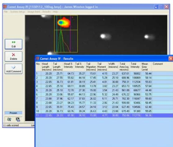
Measurements accumulated for each slide are viewable within a scrolling results window, which can be split from the main application and placed on a second screen in dual-monitor systems. The results window can also be hidden entirely for those wishing to score blind.
