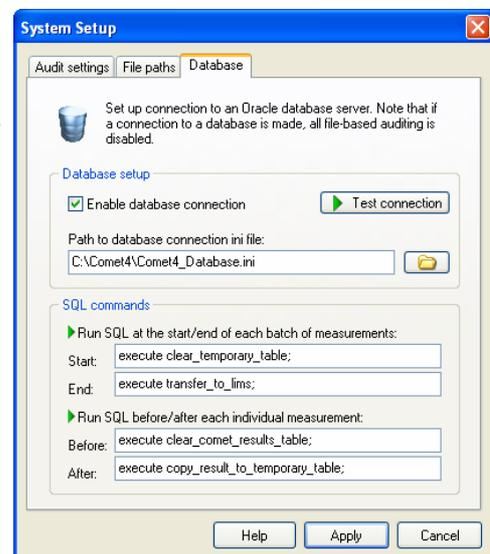
Comet Assay IV is designed to allow multiple scoring systems to connect to the same database. The database forms a secure central repository for all your data, and use of unique system and batch IDs makes it easy to identify all the data for a specific system and session of measurements.
